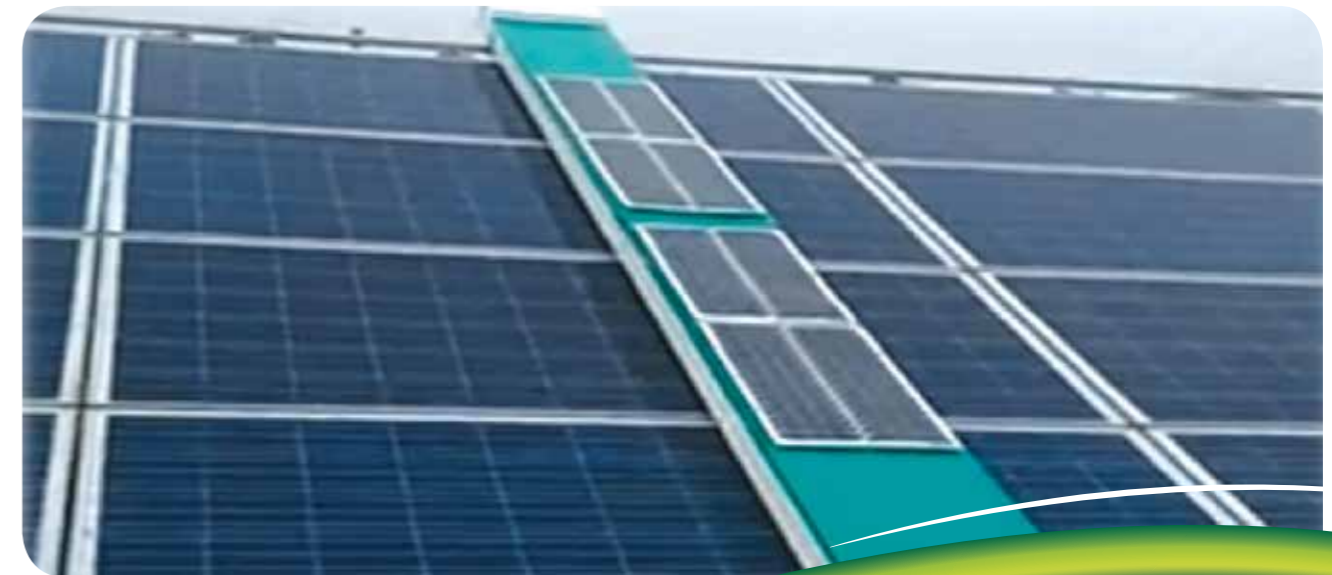
Waterless robotic solar panel cleaning system
