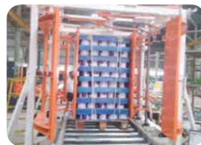
Automated pallet aligner at the Khandala factory
