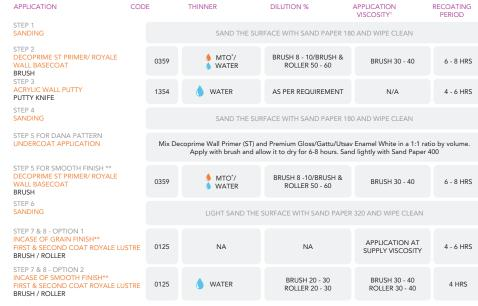
1. As measured through a Ford cup. 2. Recoat period is quoted for 25°C and 50% Relative Humidity, these may vary under different conditions. \*Mineral Turpentine Oil. \*\* Fine pattern of roller will be retained depending on type of roller used.
