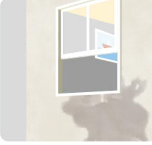
**PLASTER** New masonry surfaces must be allowed to cure completely. It is recommended to allow 28 days as the curing time for new masonry surfaces.
