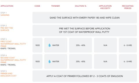
coat of Putty Prime . Also, it is recommended to prevent the surface before the 2. Recoat period is quoted for 25°C and 50% Relative Humidity, these may vary under different conditions.
